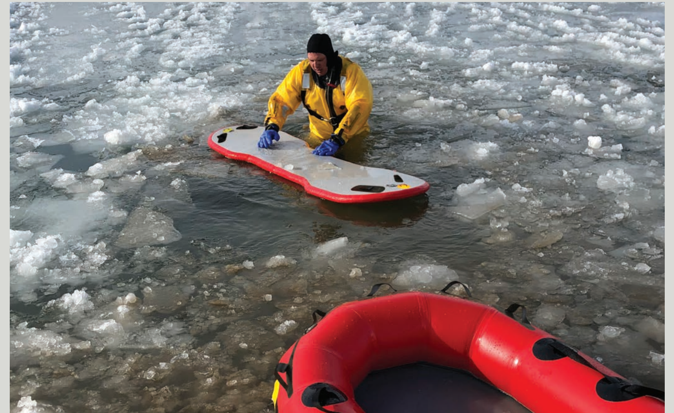
Removable / throwable floor can be used to stabilize a victim while additional rescue tools are deployed.
